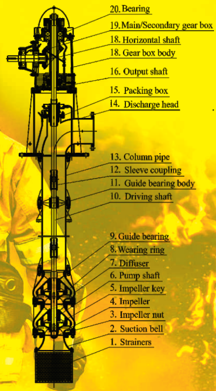
Construction Drawing (With Gear Box)
