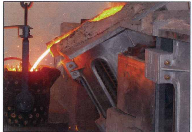
Hi-chrome iron castings being poured
