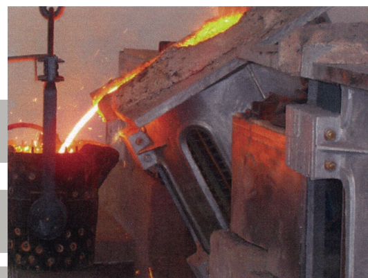
Hi-chrome iron castings being poured
